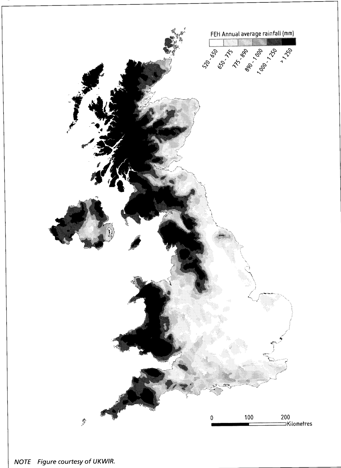
Figure 2 Hydrological regions of the UK for the sizing of rainwater harvesting systems
